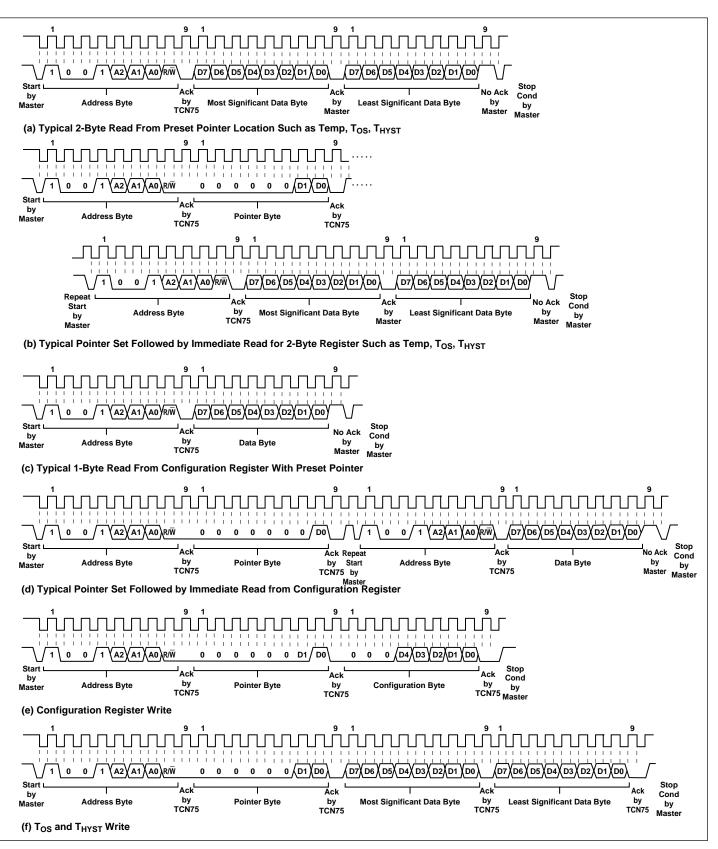
Figure 2. Timing Diagrams
